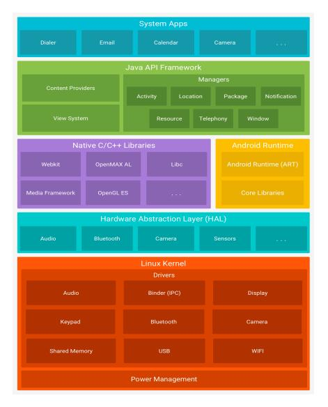
Figure 1: Android's architecture [9].
