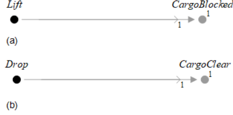
Figure 15: Guarantees 7 and 8: Dropping and lifting and the cargo sensor properties
